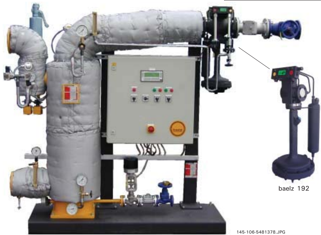
Fig. 22 typical application of the baelz 192 as emergency stop - valve and steam pressure reducing valve ahead of an steam / water heat - exchangers with condensate outlet control
